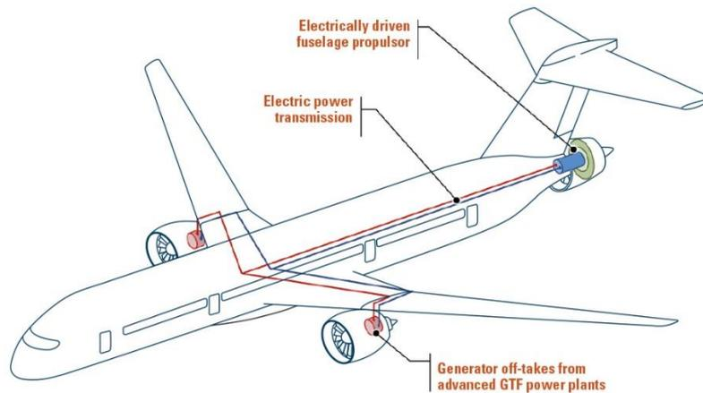
Figure 1. Overview of the PFC aircraft illustrating the power train concept [1].
