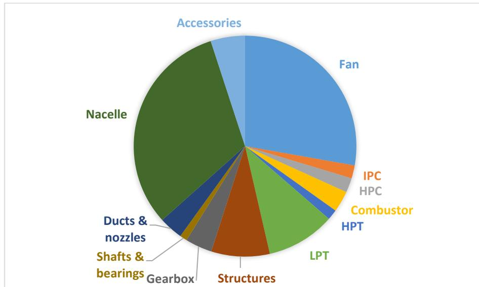
Figure 6 Component weight breakdown of the R2035 power plants. The total mass per engine is calculated to 8800 kg
