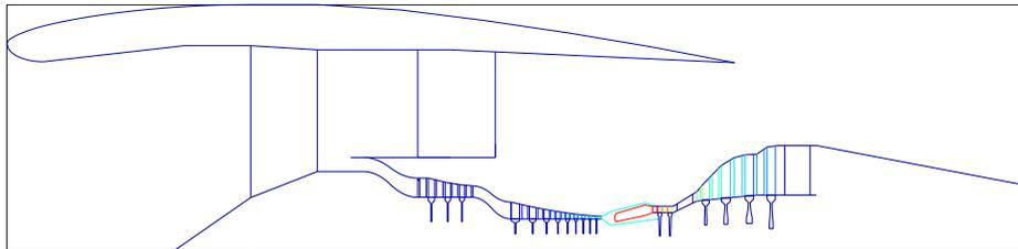
Figure 3 General arrangement and flow path layout of PFC engine
