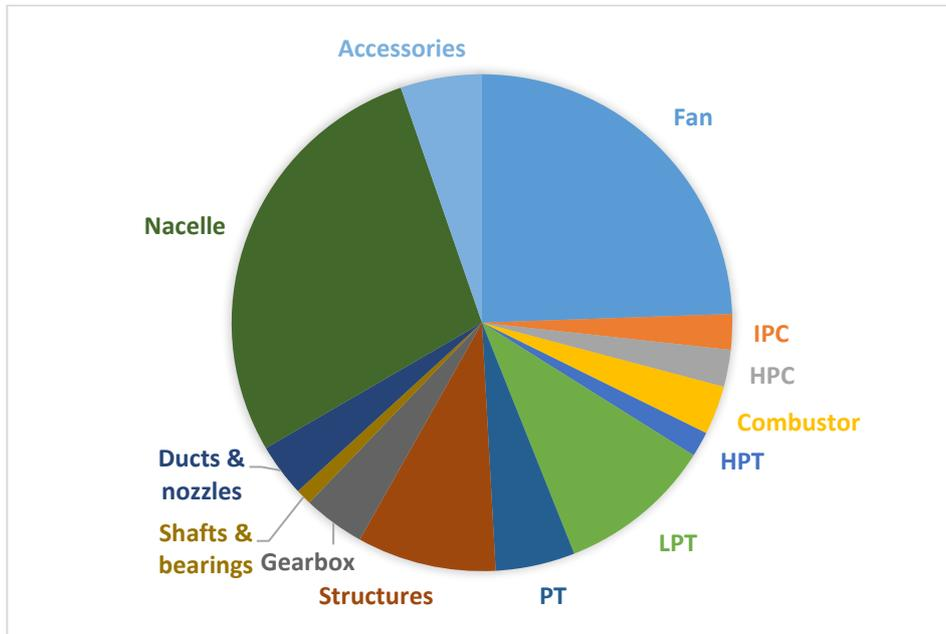
Figure 5 Component weight breakdown of the PFC main power plants. The total mass per engine is calculated to 7700 kg
