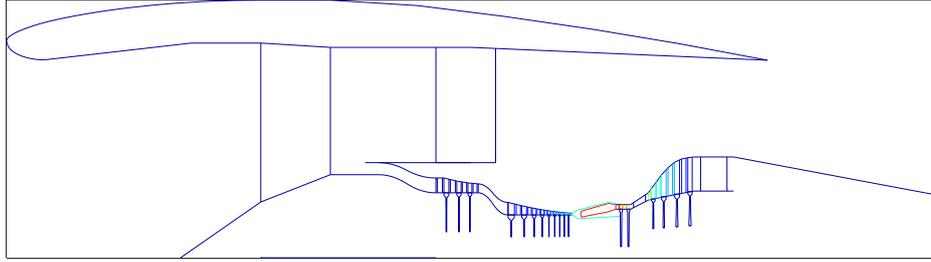
Figure 4 General arrangement and flow-path layout of the R2035 engine
