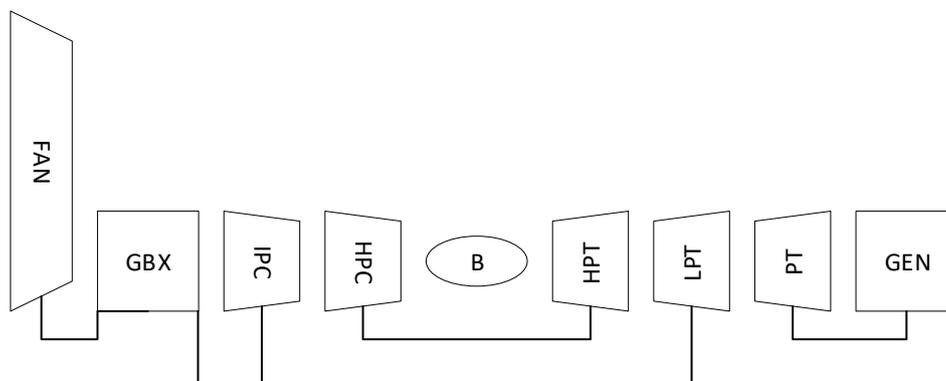
Figure 2 Schematic layout of the geared turbofan engine architecture adapted for the large power offtakes required by the PFC aircraft.
