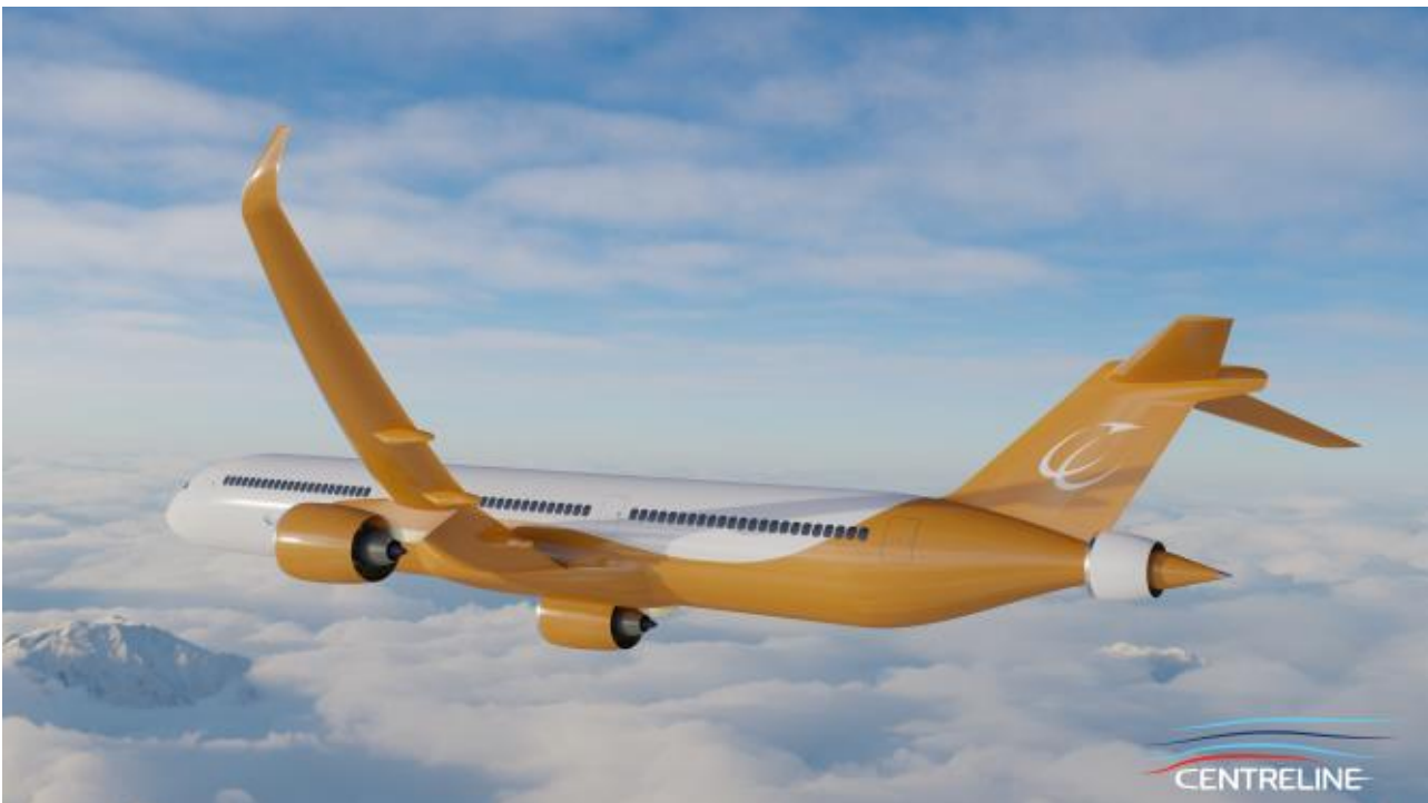
©Bauhaus Luftfahrt e.V. CENTRELINE turbo-electrically driven fuselage wake-filling aircraft
